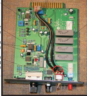
Massive polyester input decoupling capacitors
